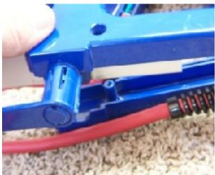
Make sure that this peg lines up with the hole on top! Replace that screw first, as it is the one that holds the metal bar in place, then replace the other screws. Make sure the switch is turned off, and plug the machine back in and make sure it works.
