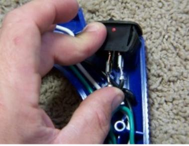
Making sure that all of the wires are in their proper channels, nooks and crannies, carefully place the top half of the handle back on the bottom half, as in the next picture.
