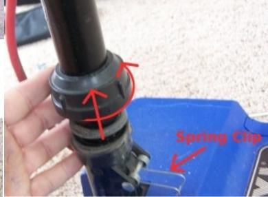
Locate the clog, either in the tube or in the base of the vacuum, and clear it out. Replace the tube, filter bag, dock, and dust bag. As long as it is taken apart, you might as well take the filter (cloth) bag outside and clean it according to the regular maintenance section later in this manual.
