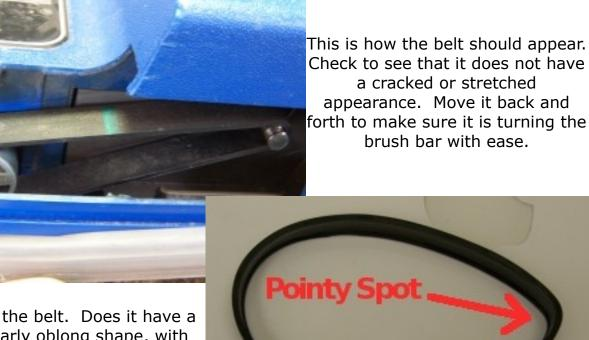
Remove the belt. Does it have a particularly oblong shape, with one spot in particular that is pointier than the rest? This is the spot where the motor pulley was rubbing against the belt.
