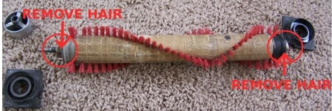
Replace the plastic brackets and screw the pulley back on (counter-clockwise!) Replace the brush with the brackets in the same position and put the belt back. Turn the brush a few times to straighten the belt, and replace the bottom plate.
