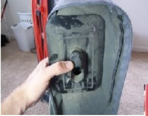
And gently pull the tube straight up from the base of the vacuum:
