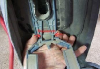
Sqeeze the hinge of the dock together to remove the bag attachment.
