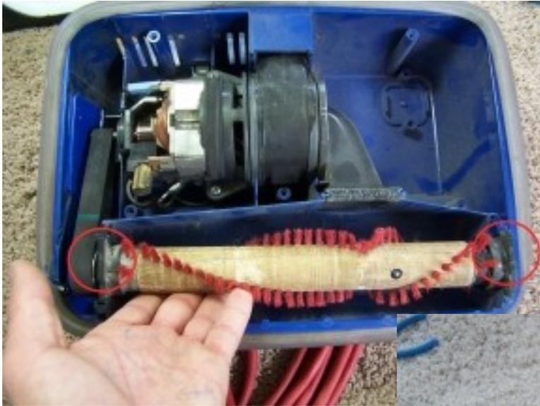
Gently remove the bottom plate, keeping track of the 5 screws.
