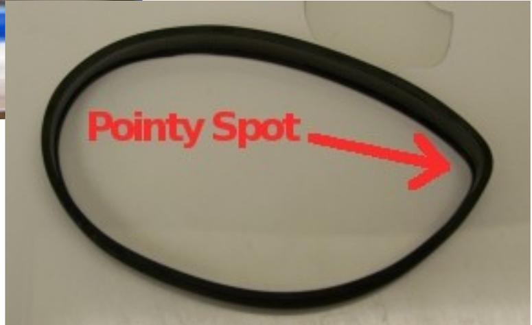
This is the most common belt problem and is caused by thick carpet, full bags, or dirty bearings on the beater bar. Replace the belt and move on to burning hair symptoms.
