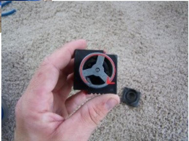
Use a pair of pliers, razor blade, or knife to remove as much hair out from underneath the bearings as possible. If necessary, the bearings can be removed by carefully prying them straight out from the brush.
