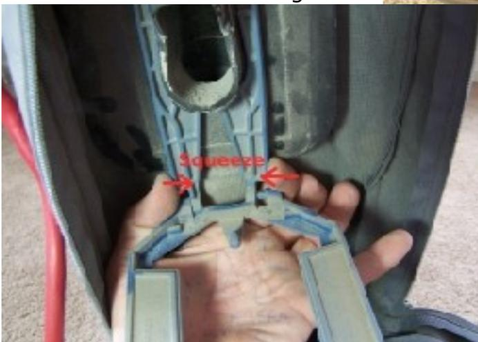
Squeeze the hinge of the dock together to remove the bag attachment.
