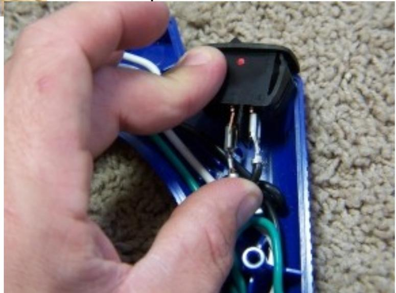
Make sure it is firmly attached! If you have a pair of needle-nose pliers, squeeze the spade just slightly to make the fit tighter.
