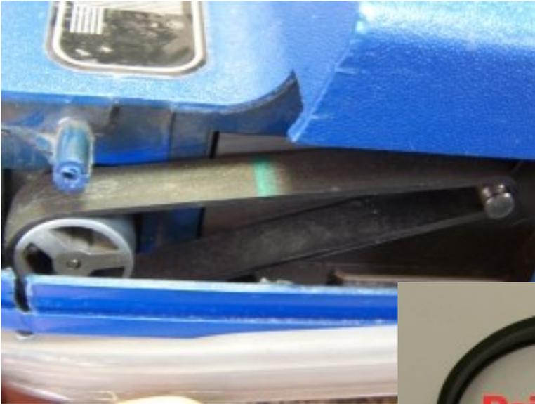
This is how the belt should appear. Check to see that it does not have a cracked or stretched appearance. Move it back and forth to make sure it is turning the brush bar with ease.
