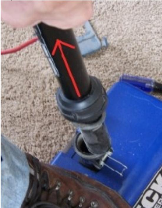
Locate the clog, either in the tube or in the base of the vacuum, and clear it out. Replace the tube, filter bag, dock, and dust bag. As long as it is taken apart, you might as well take the filter (cloth) bag outside and clean it according to the regular maintenance section later in this manual.
