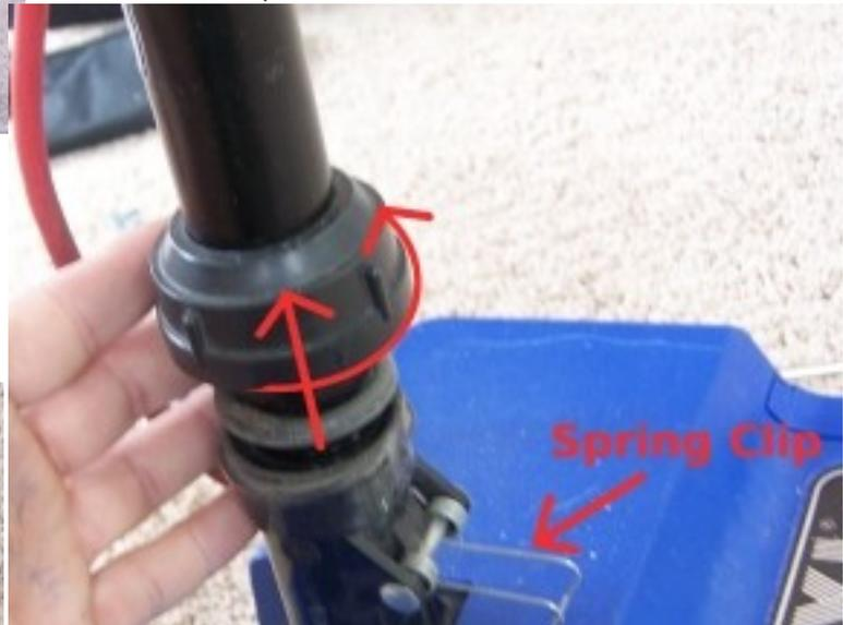
And gently pull the tube straight up from the base of the vacuum:
